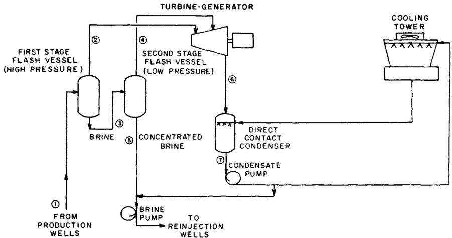
Fig. 50.6 Two-stage flash conversion.
